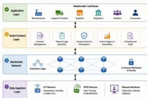
Figure 1: Four-Layer Architecture of the Blockchain-Based Supply Chain Management Framework
